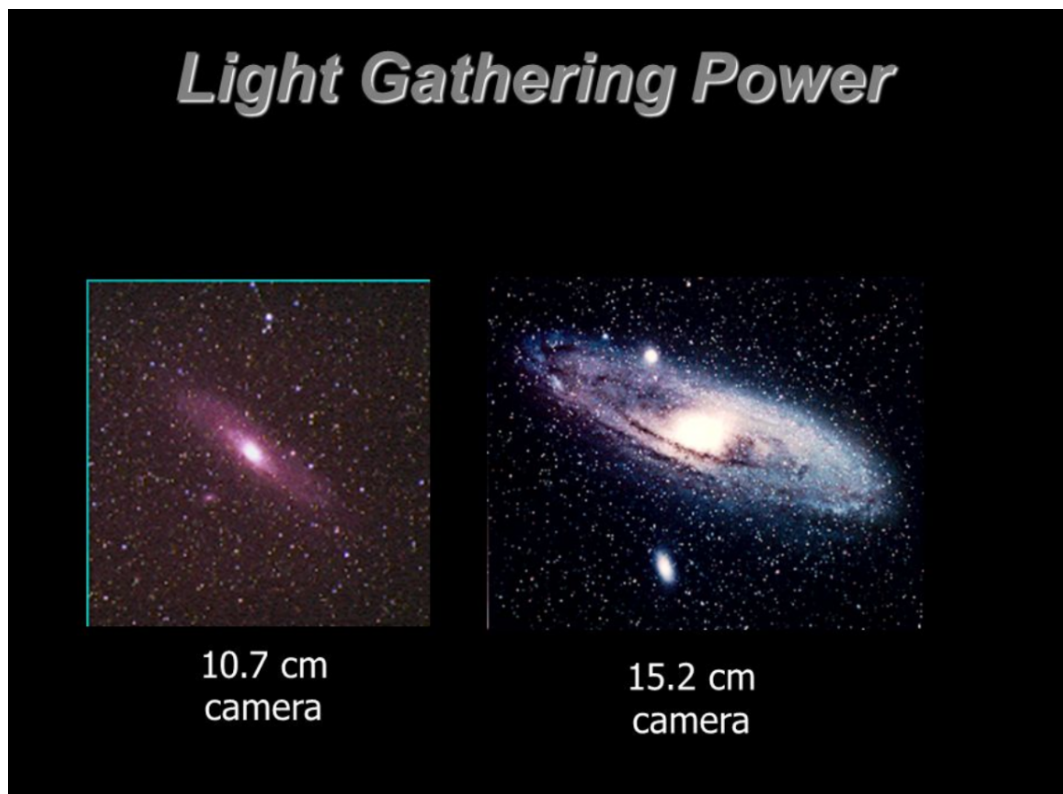
Figure 4.3: Aperture and the light gathering power
